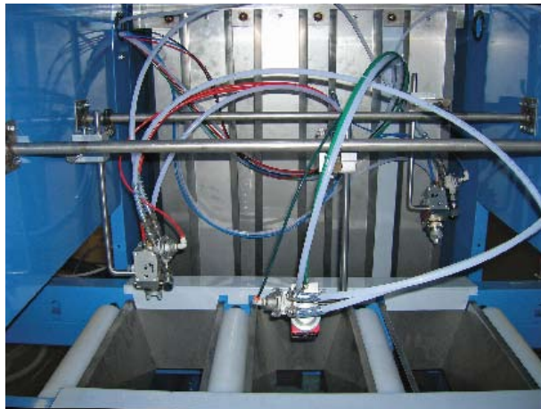
Deimco pre-baffle style spray enclosure for product reclaim — Stainless Steel Baffle
