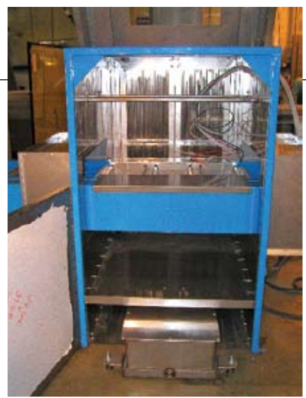
Stainless Steel capture tank with pump outlet for pumping reclaim material to filter — MFM Capture Tank
