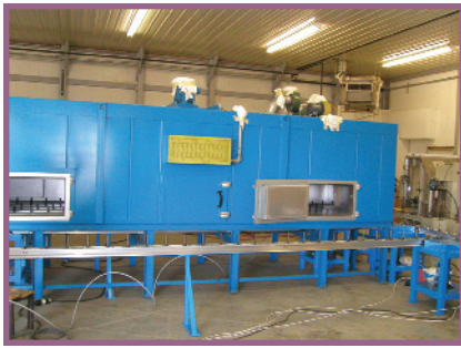
Figure 9: COE liquid cell with convection oven for heat-sensitive substrate.
