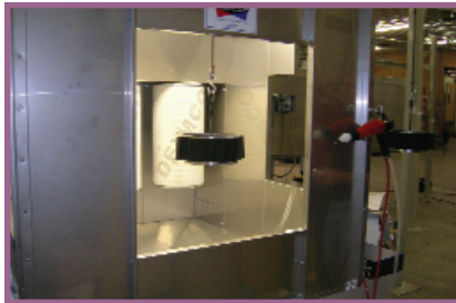
Figure 12: Lean cell with manual spray powder booth.
