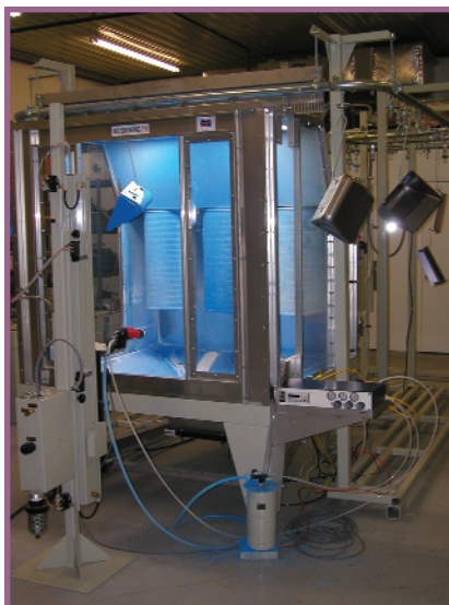
Figure 6: Lean powder cell with automatic gun and gun mover.
