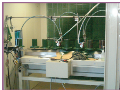
Figure 1: COE lean liquid cell with one part per fixture on eight-in. centers.
