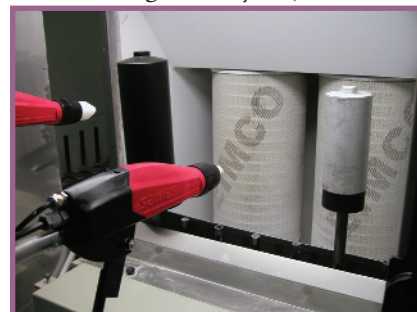
Figure 7: COE lean cell powder booth with automatic guns and powder reclaim.
