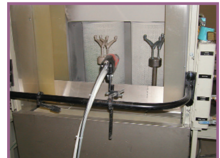
Figure 2: COE lean powder cell with four parts per fixture on 12-in. centers.
