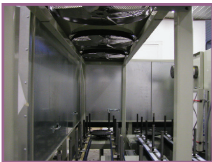
Figure 10: COE lean powder cell cooling section.
