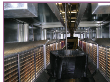
Figure 8: A 100-pound powder coated part curing in a lean cell IR oven.
