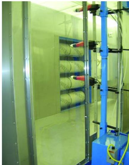
those parts are triggered. Due to the large coverage area and fan pattern of an automatic gun, high-resolution part detection systems using light curtains are typically an unnecessary expense.
